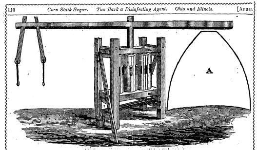
are a sufficient distance apart to admit of the rollers and the frame work that supports and confines them to stand altogether within them; this gives room for the trough underneath, which catches the whole of the juice ; the edge of this trough can be seen as ning out at the end into a bucket. Every thing else will be found sufficiently explained in the Report less offensive. above referred to.
