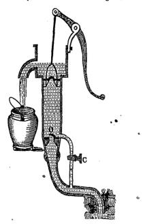
is merely a metalic tube, with two valves—the first attached to the handle, and represented as shut; the second made stationary at O, and represented as open. Supposing the pump empty, and the end of the handle elevated, the tube will of course be full of air. On lowering the handle, the upper
