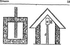
preventing the ingress of damp or heated atmosphere from without. There ought also to be small apertures through the walls on opposite sides for ventilation in dry or cool weather and which can be perfectly shut when the air is damp.
