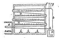
"The above figure will give a general idea of the apparatus. It consists of a square box of any required size. A small furnace is seen at a, furnished with a boiler. From this arises a tube, b, which traverses backward and forward through the box, and through another one which is partly shown at e, where the chickens are kept after being hatched, and returns into the boiler, a. The eggs rest on the shelves, c.
